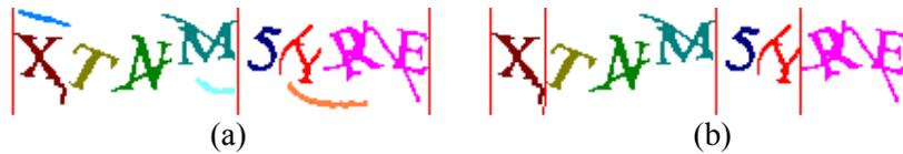
**Fig 11. Arc removal - relative position checking. As shown in (b), further arcs in (a) are removed and histogram is updated.**
